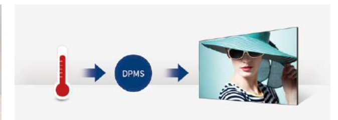
As it is designed to enter DPMS (display power management signaling) mode automatically whenever the temperature of display is detected to be higher than a certain limit, it prevents damage from overheating by long-term use or radiant heat in advance.
